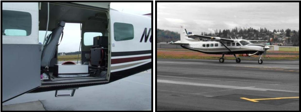
*The Cessna Caravan is a stable platform, ideal for flying slow and low for high density projects. A Leica ALS50 sensor head installed in the Caravan is shown on the left.*
