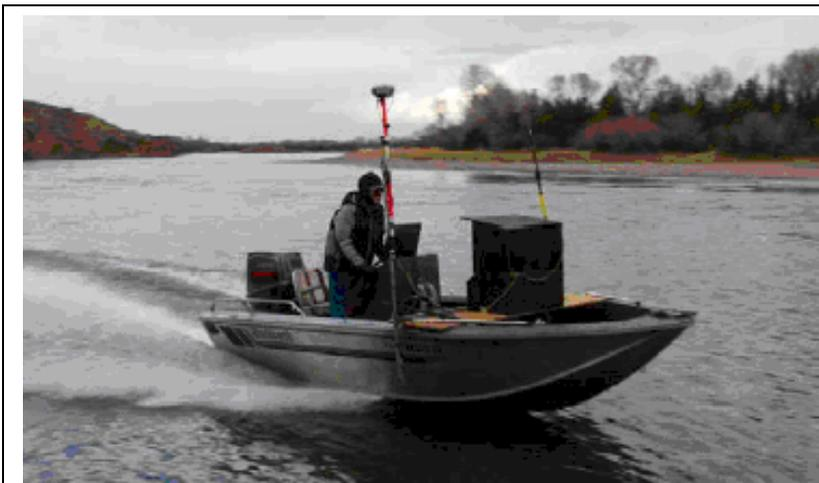
*Figure 13* - Survey Vessel used for the Missouri River Bathymetric Survey. The Trimble R8 antenna is located on top of the red sonar mast.
