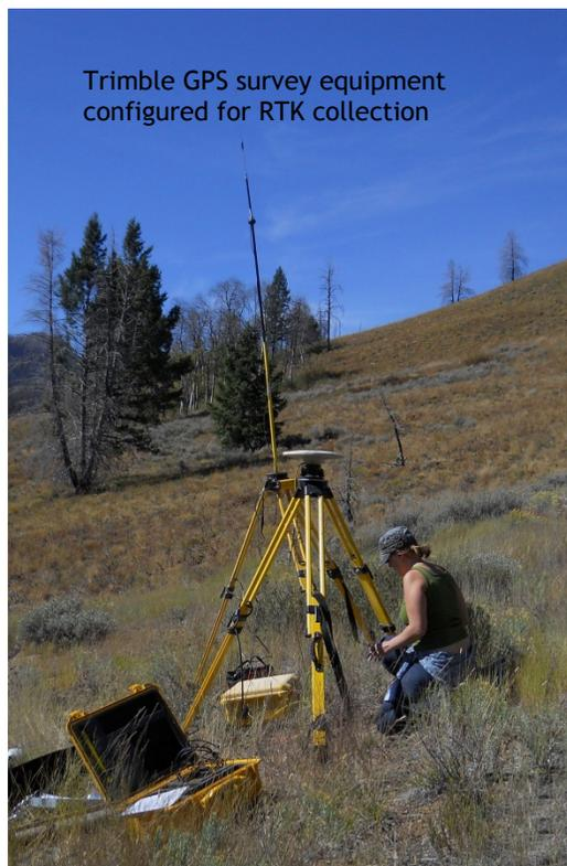
Trimble GPS survey equipment configured for RTK collection
