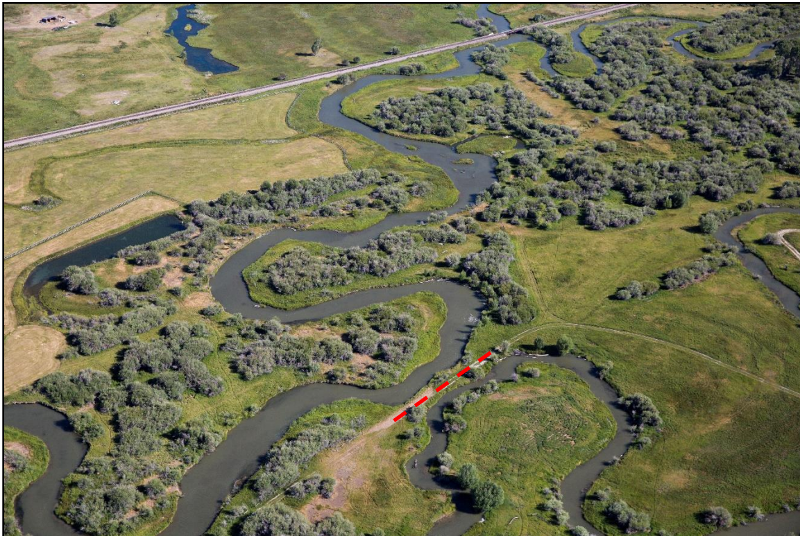
Figure 49. View downstream showing potential avulsion site between Beaverhead River (left) and Poindexter Slough (right). (Kestrel)
