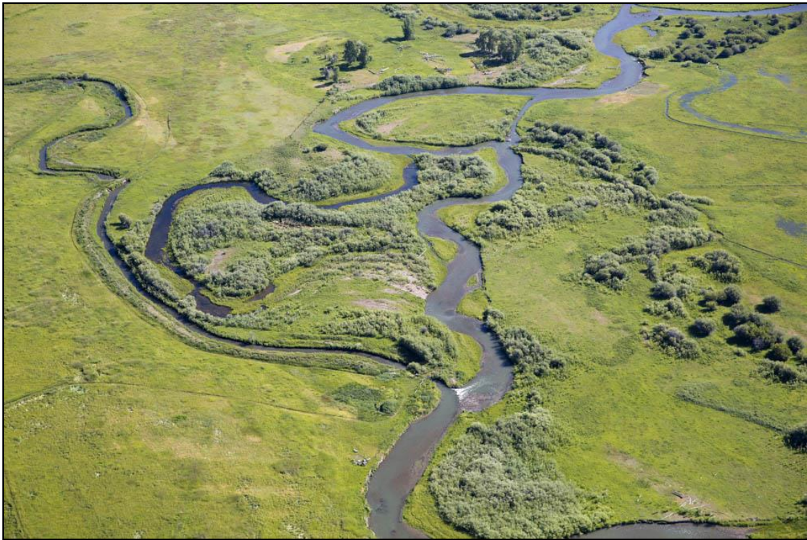
Figure 56. View downstream showing area of 1979-2013 avulsion and active chute channel cutoff just beyond, RM 40.9. (Kestrel)
