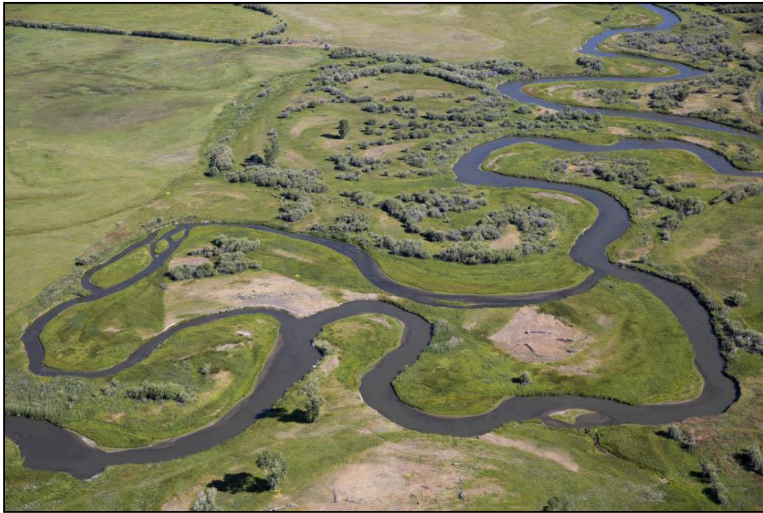
Figure 61. View downstream showing area of imminent cutoff (center of photo), RM 24.7. (Kestrel)
