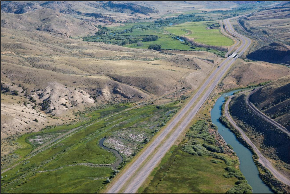
Figure 42. View downstream below Clark Canyon Dam showing 1955 meander isolated by interstate bridge and major landslide crossing river valley just downstream. (Kestrel)
