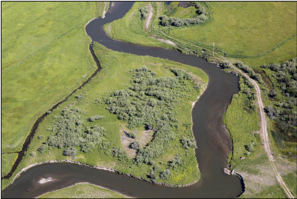
Figure 69. View downstream showing potential avulsion route through ditch, RM 3.4. (Kestrel)
