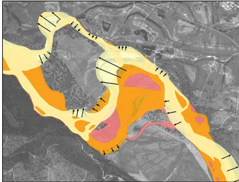
Figure 8. 2005 air photo and digitized bankfull polygons showing migration vectors, Reach 4 near Frenchtown (Pink=1955, Orange = 1972, and Yellow = 2005).
