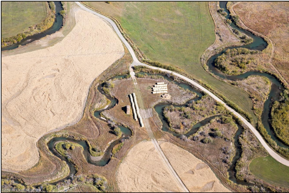
Figure 14. Intermittent bank armor on Clear Creek associated with roads, bridges, and fields. (Kestrel)
