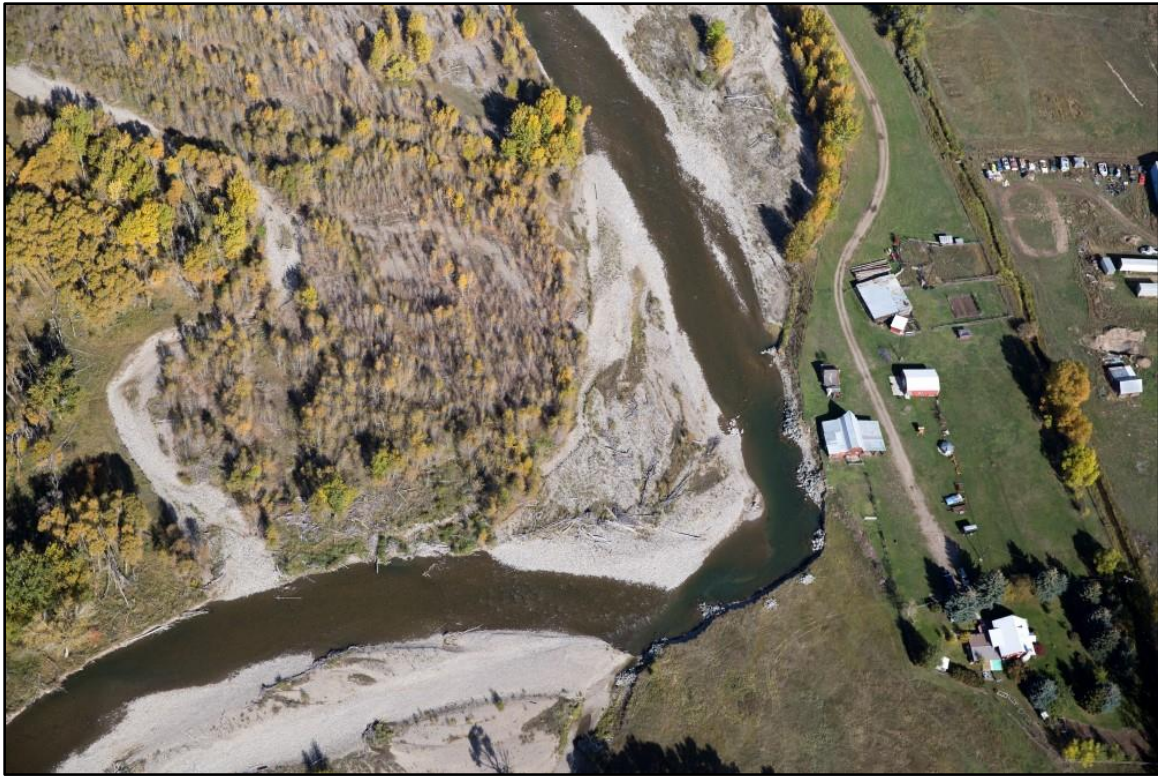
Figure 59. Barn on right bank where river has migrated 216 feet since 1965, RM 23.2 (Kestrel).
