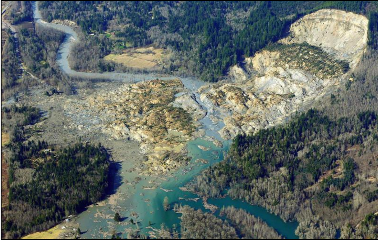
Figure 11. Massive mudslide in Oso Washington on March 22, 2014, deflecting the North Fork of the Stilliguamish River (AP Photo/Ted Warren).
