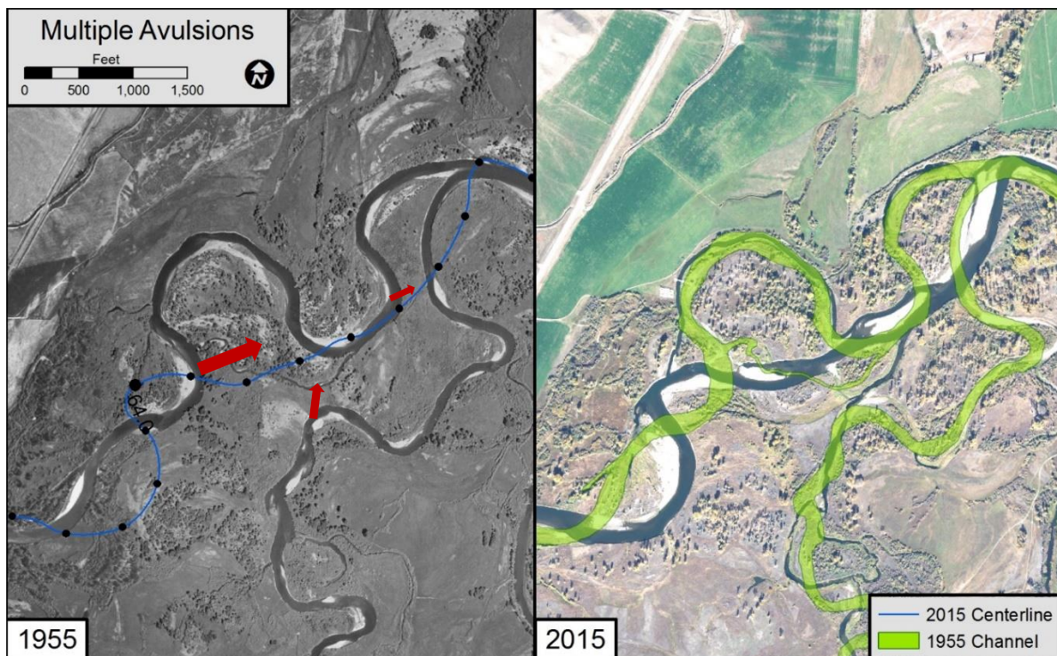
Figure 48. Imagery from 1955 (left) and 2015 (right) showing three avulsions and resulting channel straightening below Silver Star.
