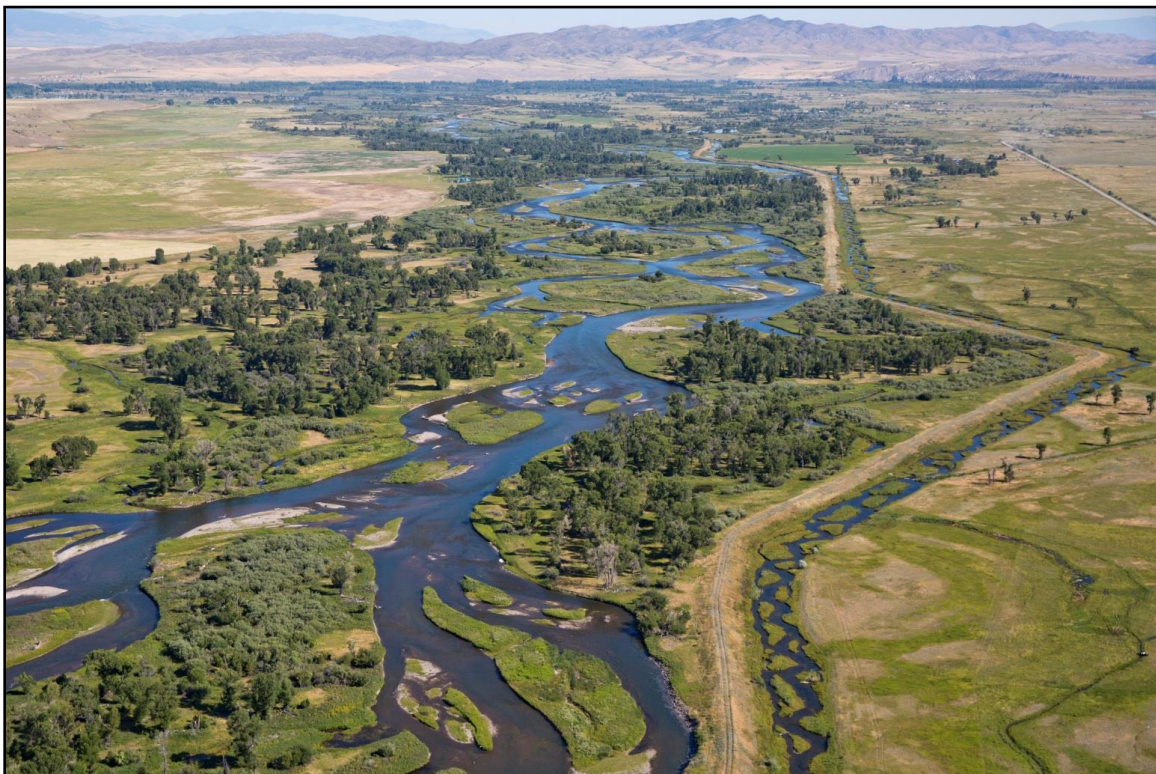
Figure 21. The Madison River south of Three Forks on July 21, 2016, showing the 10.6 mile long Madison River Levee. Darlington Ditch follows the landward side of the levee. (Kestrel)
