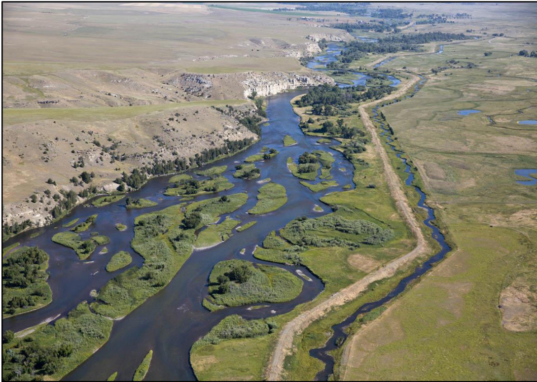
Figure 61. View downstream showing Lower Madison Levee confinement on east bank, with Darlington Ditch flowing on the right (landward) side of the levee. (Kestrel)
