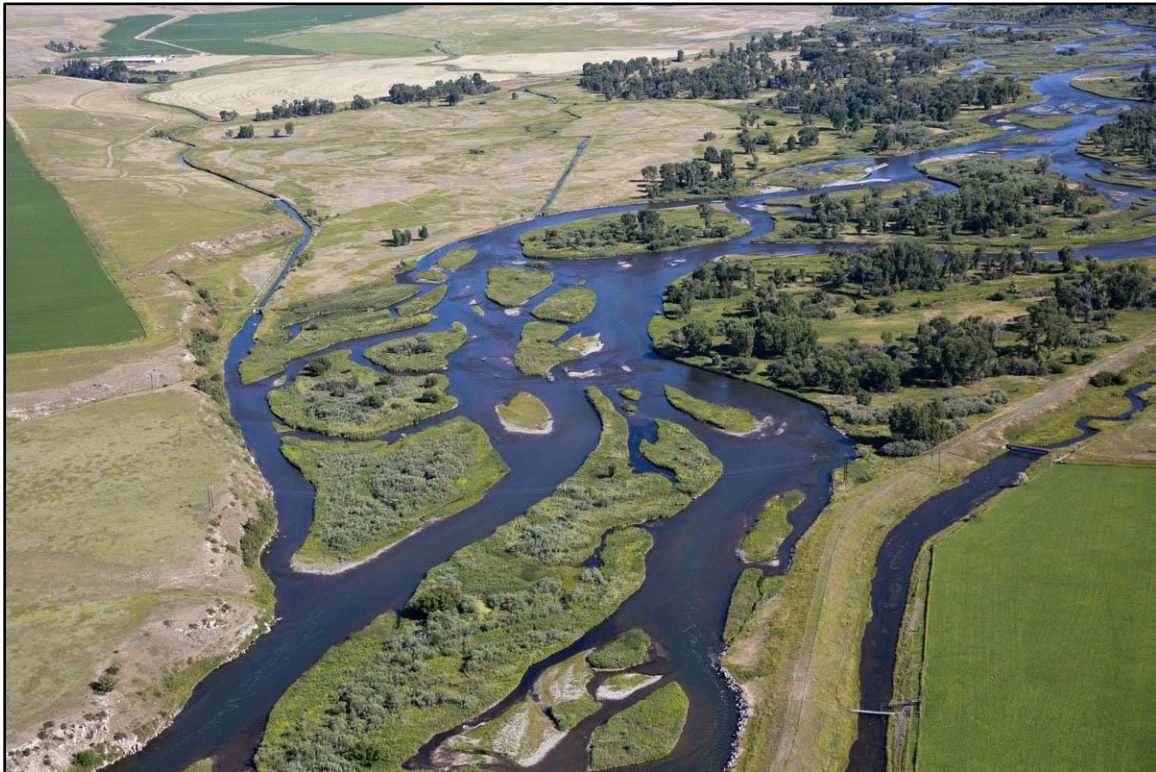
Figure 63. View downstream showing armored levee on right bank at pinch point (foreground). (Kestrel)
