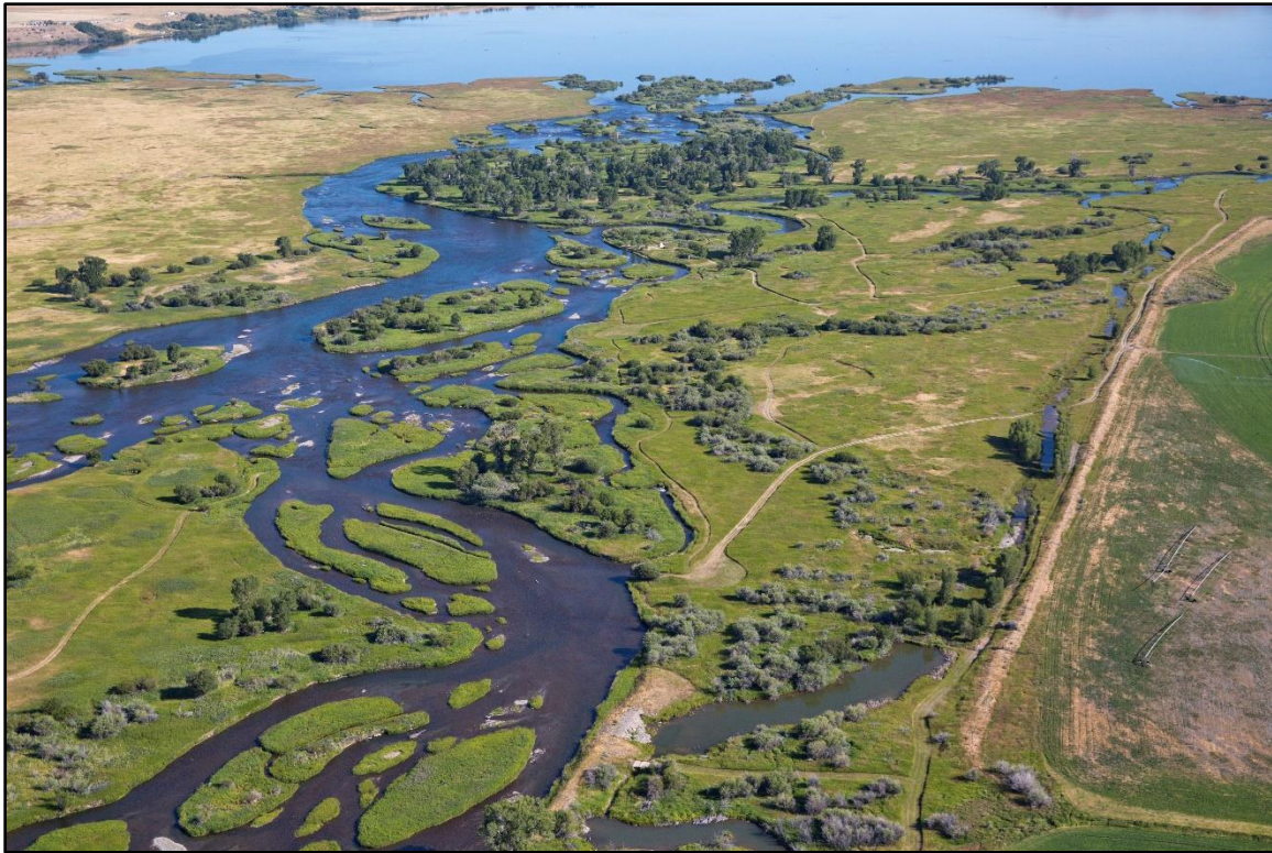
Figure 52. View downstream showing 1955-1979 avulsion blocked by channel plug in foreground. (Kestrel)
