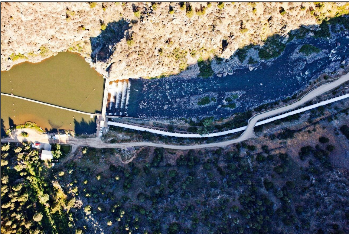
Figure 54. Sediment-starved channel form below Madison Dam. (Kestrel)
