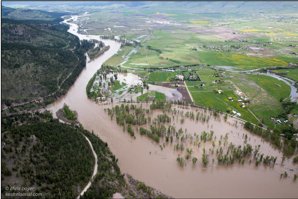
Figure 86. View downstream of Reach CF09 during 2018 flood; note Harpers Bridge Road acting as a levee in right foreground (May 10, 2018).
