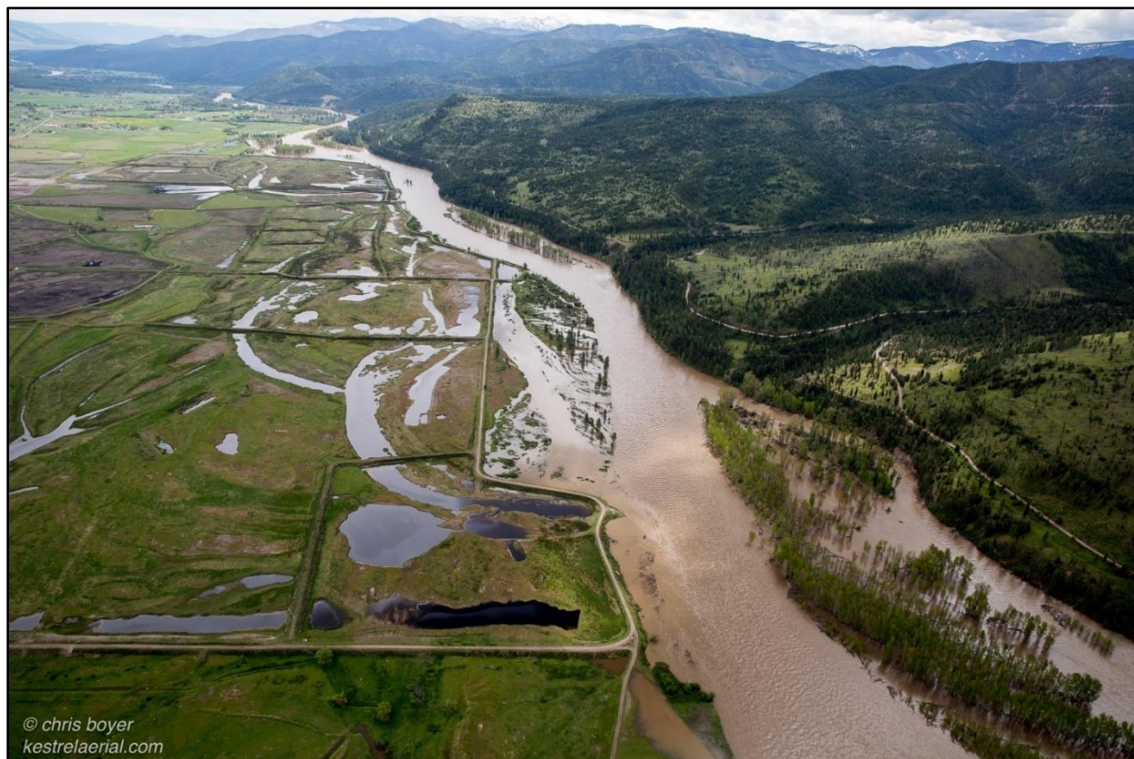
Figure 88. View upstream showing Smurfit Stone dike system that confines river to narrow corridor against the bluffline to right (May 10, 2018).
