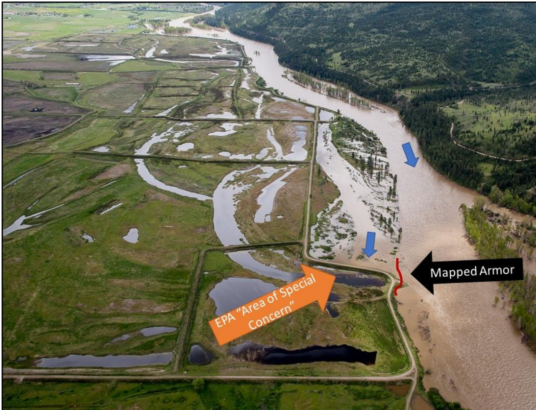
Figure 119. View upstream of armor at RM 196.15 showing flow behind treatment hitting Smurfit Stone berm at right angle.
