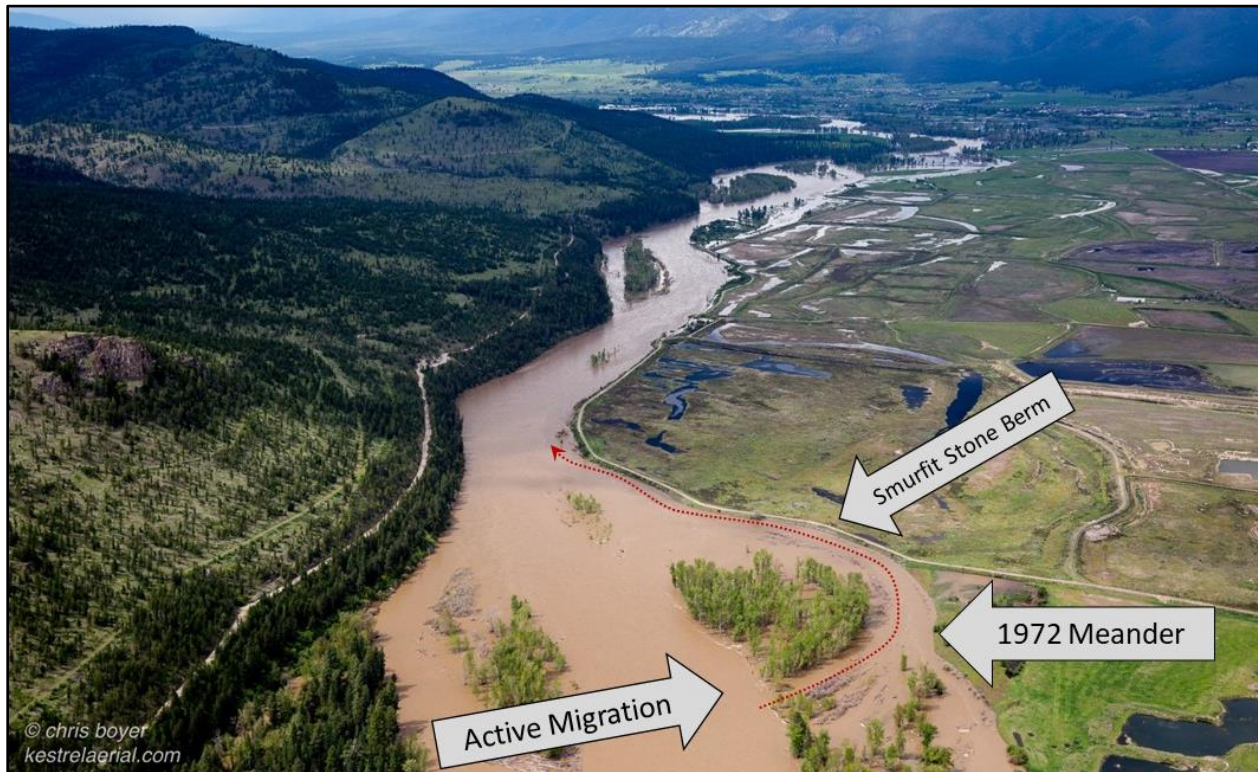
Figure 114. 2018 flood photo showing high flow activation of meander swale that flows against Smurfit Stone berm at upper end of mill site (May 10, 2018).
