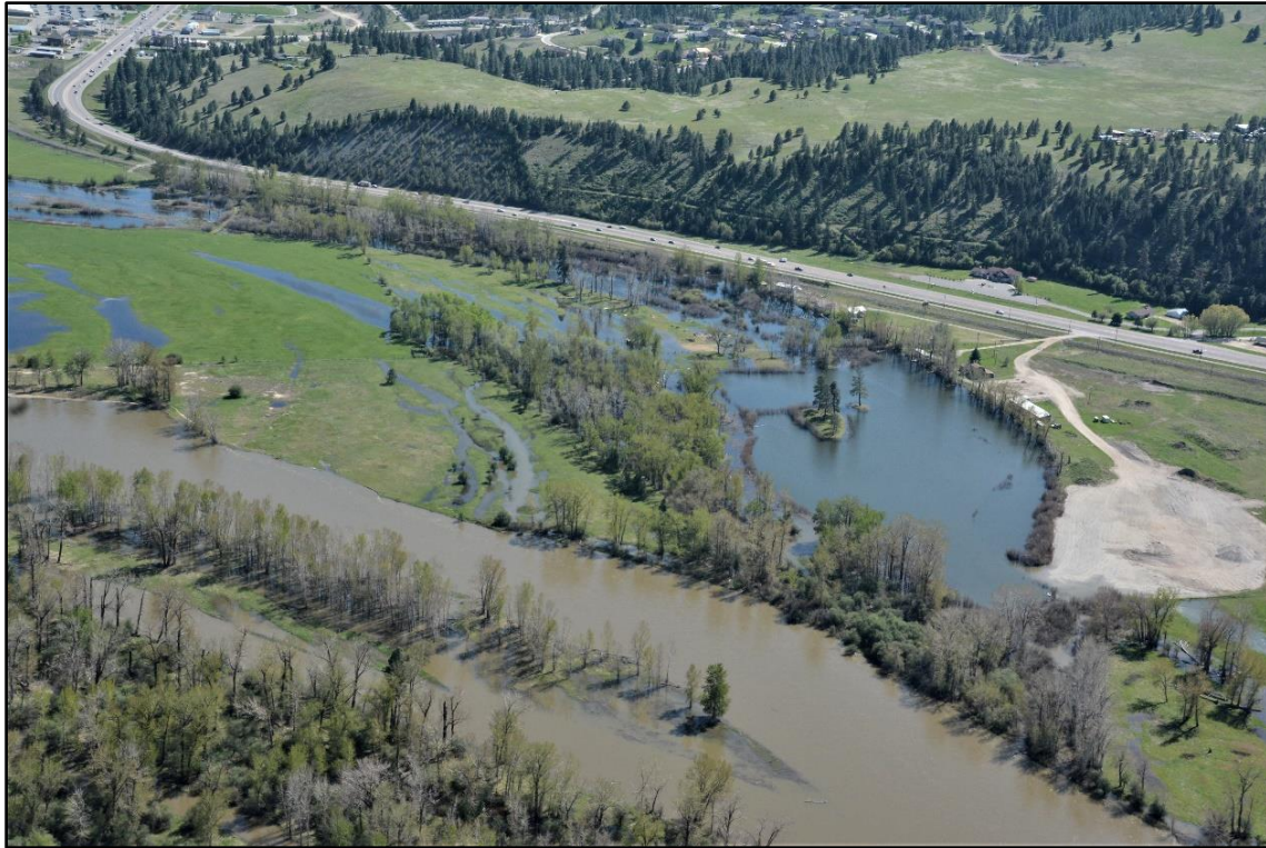
Figure 100. View upstream showing lower end of flooded swale below water treatment plant; migrating bank follows the vegetated strip between swale and river (CAP May 8, 2018).
