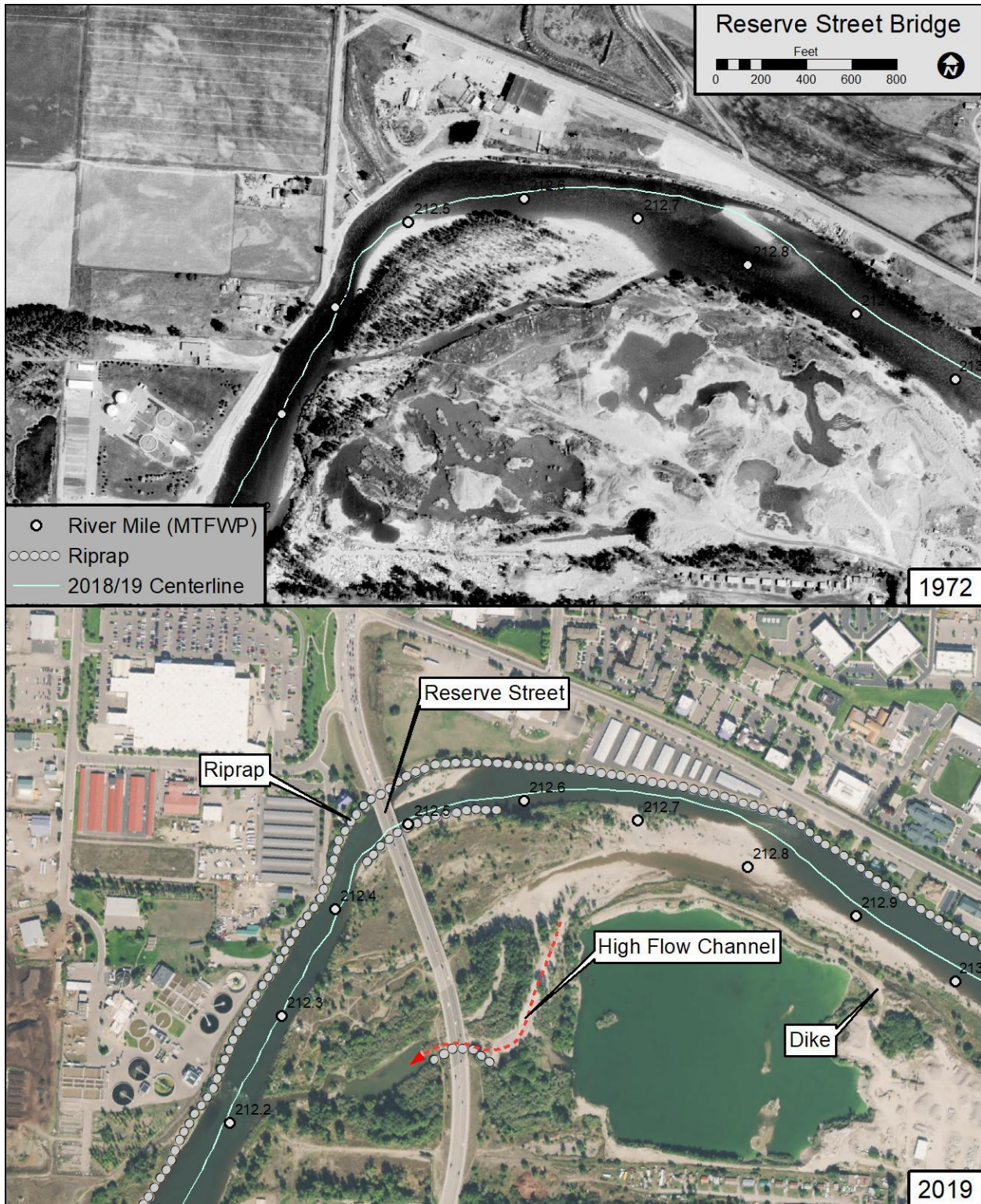
Figure 64. Gravel pit and high flow channel development at Reserve St Bridge, 1972 (top) and 2019 (bottom).
