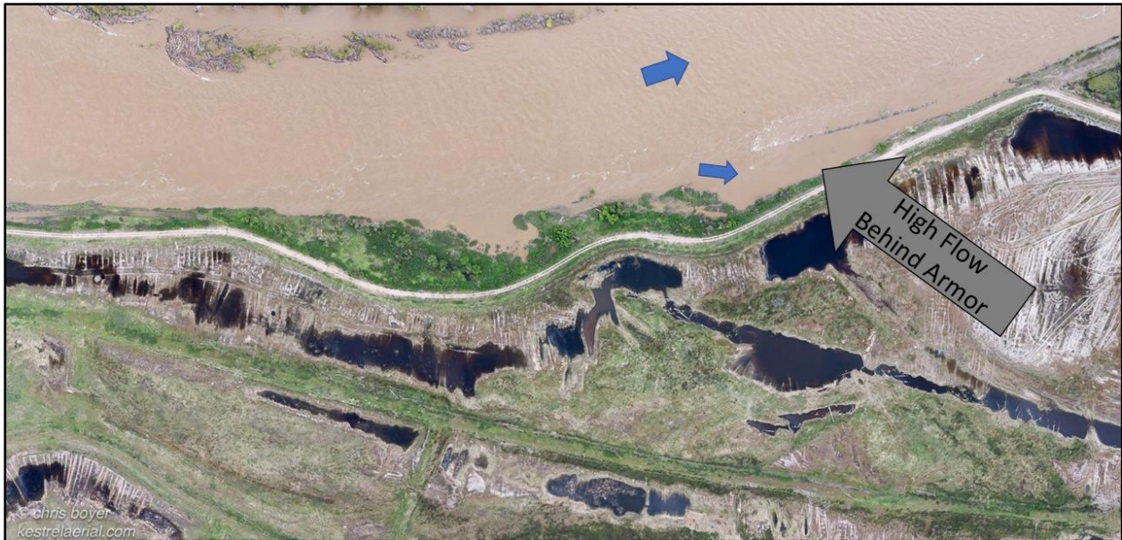
Figure 116. 2018 flood photo of bank armor at RM 197 (Pond #11) showing linear rock treatment largely submerged; note high flow velocities visible on upper end of treatment.
