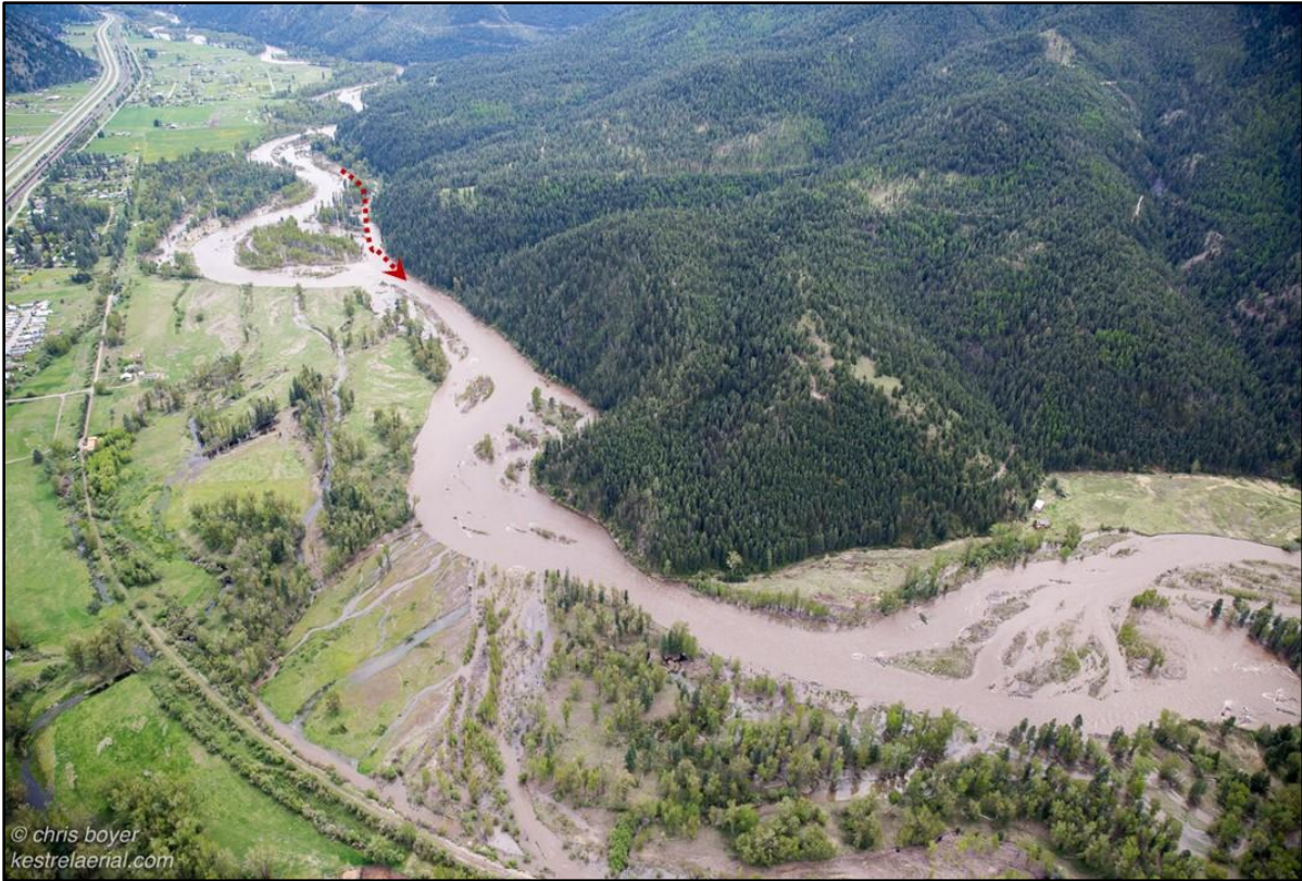
Figure 51. View upstream during 2018 flood showing channelized overflow into floodplain swales in foreground, RM 233. The large meander in the upper left portion of photo fully cut off by the end of the flood (avulsion path shown in red).
