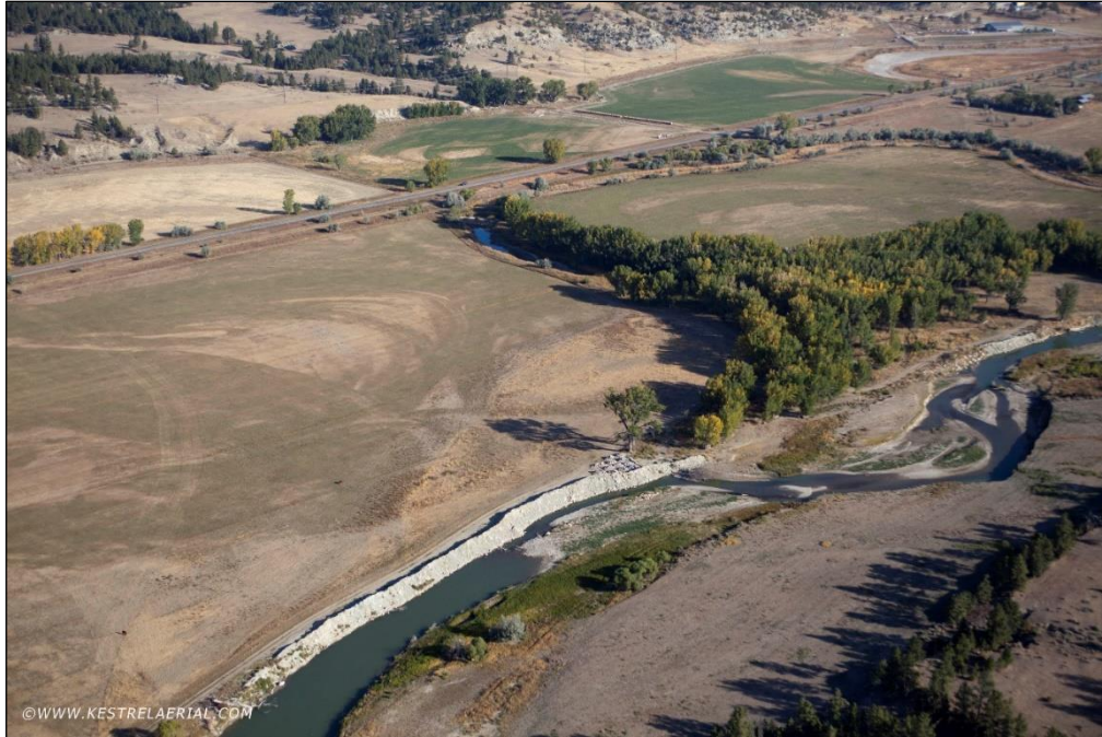
Figure 26. View downstream showing left bank armoring just below Goulding Creek Road Bridge (Sept 20, 2012, Kestrel).
