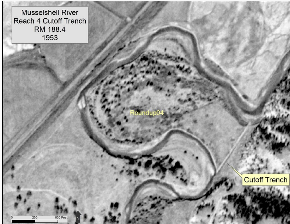
Figure 24. 1953 image at RM 188.4 showing cutoff trench excavated through meander core.
