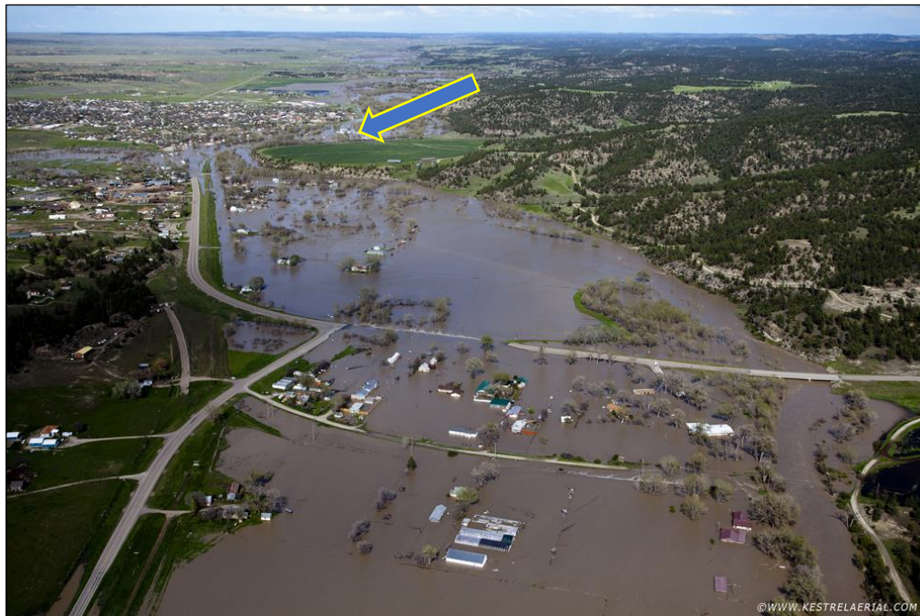
Figure 32. View downstream of bedrock constriction (arrow) at Roundup during 2011 flood (May 26, 2011—Kestrel).
