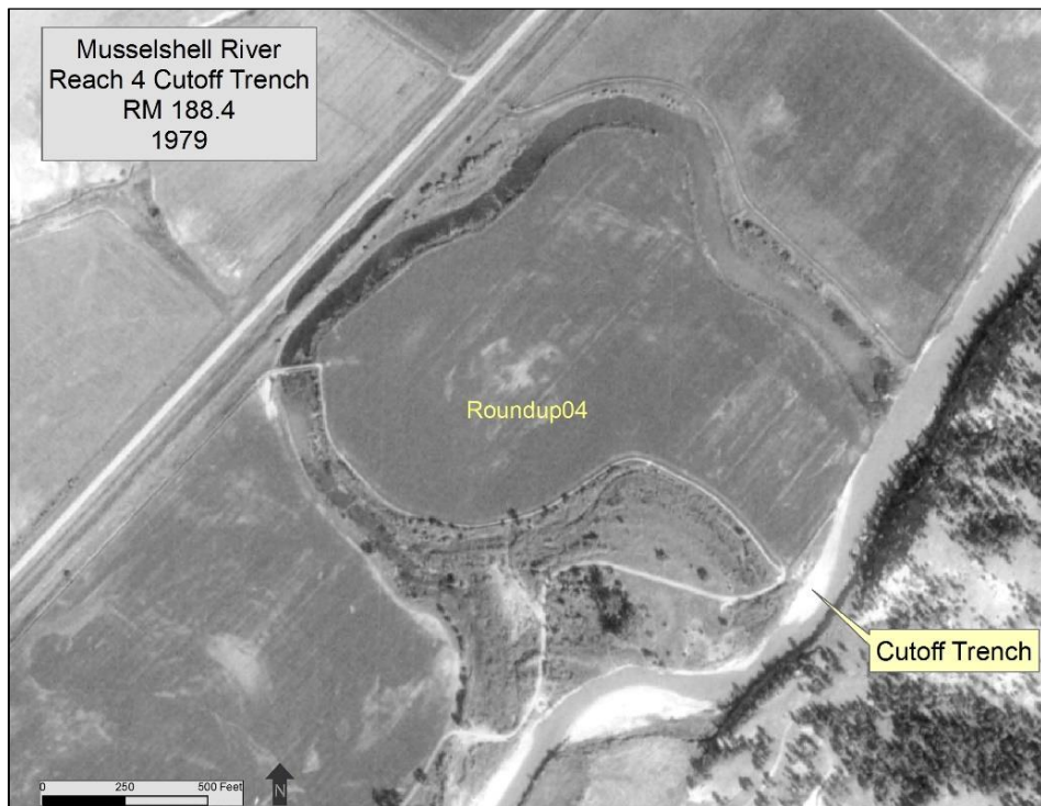
Figure 25. 1979 image at RM 188.4 showing trench capture of main river channel.
