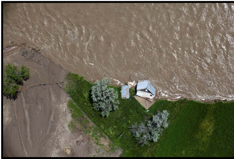
Figure 2. A home falls into the Musselshell River in June 2011 after the river migrated and undermined its foundation. (©www.kestrelaerial.com)
