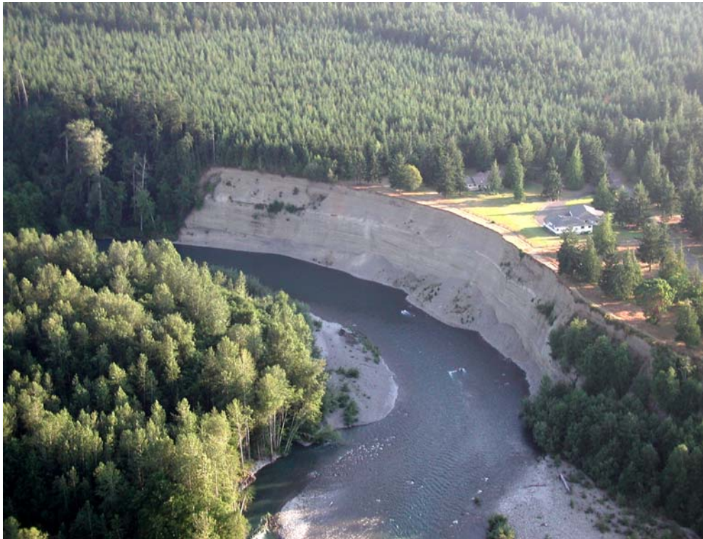
Figure 16. An eroding terrace bank along the western margin of the lower Elwha River, looking upstream (July 2002). The terrace bank is composed of glacial outwash. Despite a height of ~41 m, the Elwha River actively erodes this bank and causes chronic mass wasting and instability. Because the river has sufficient transport capacity to remove all materials eroded from the bank, its vertical slope is maintained by the river's position along its toe. If the Elwha River migrates away from the toe of the terrace bank, a flatter slope angle will develop as mass wasting establishes a more stable configuration, thereby causing further retreat of the bank top.
