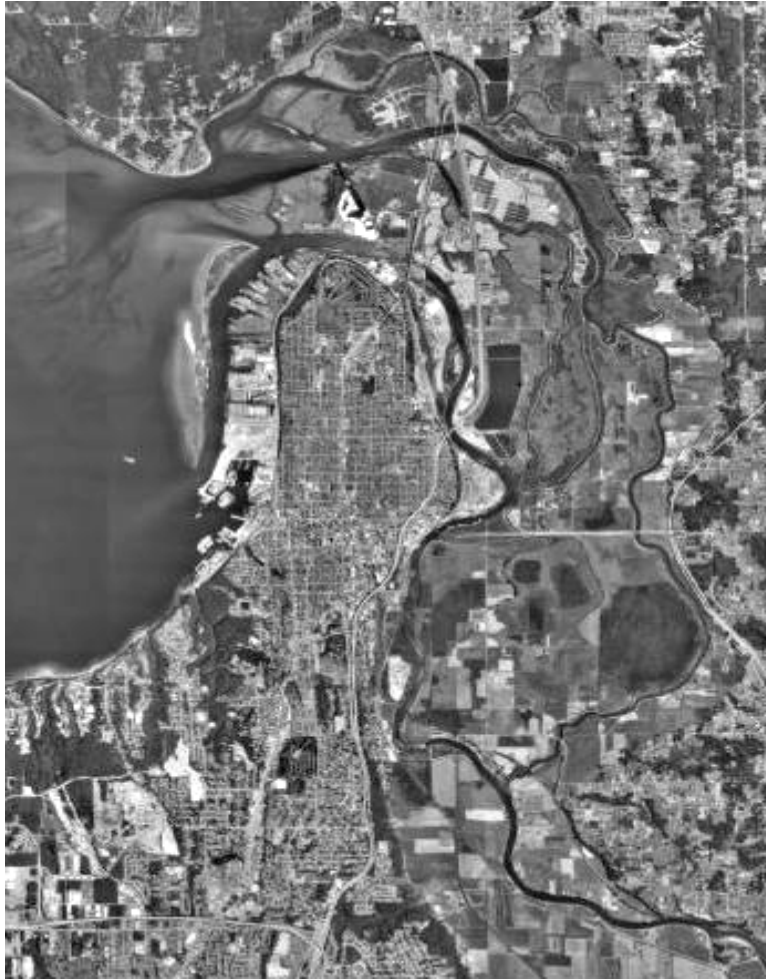
Figure A-6. A highly altered deltaic distributary channel; Snohomish River, Everett, WA. Aerial photo 1990.
