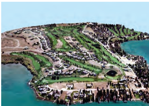
bottom image is derived from orthophotographs draped over digital surface model.
