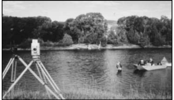
17. USGS-WRD team conducting cross-section survey. Photo courtesy of USGS.
