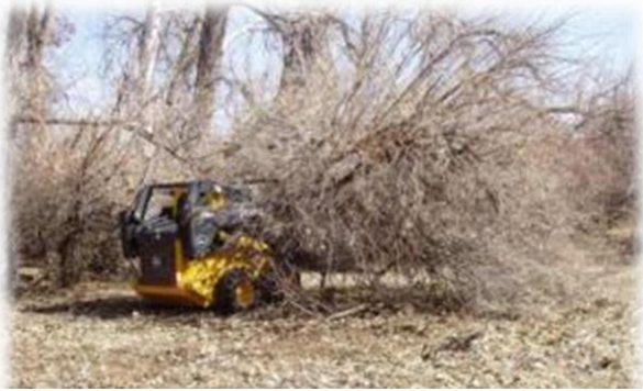
Figure 3. Motorized shears cut and remove large, mature Russian olive understory prior to cut stump treatment. Photo Credit: USDA-ARS.
