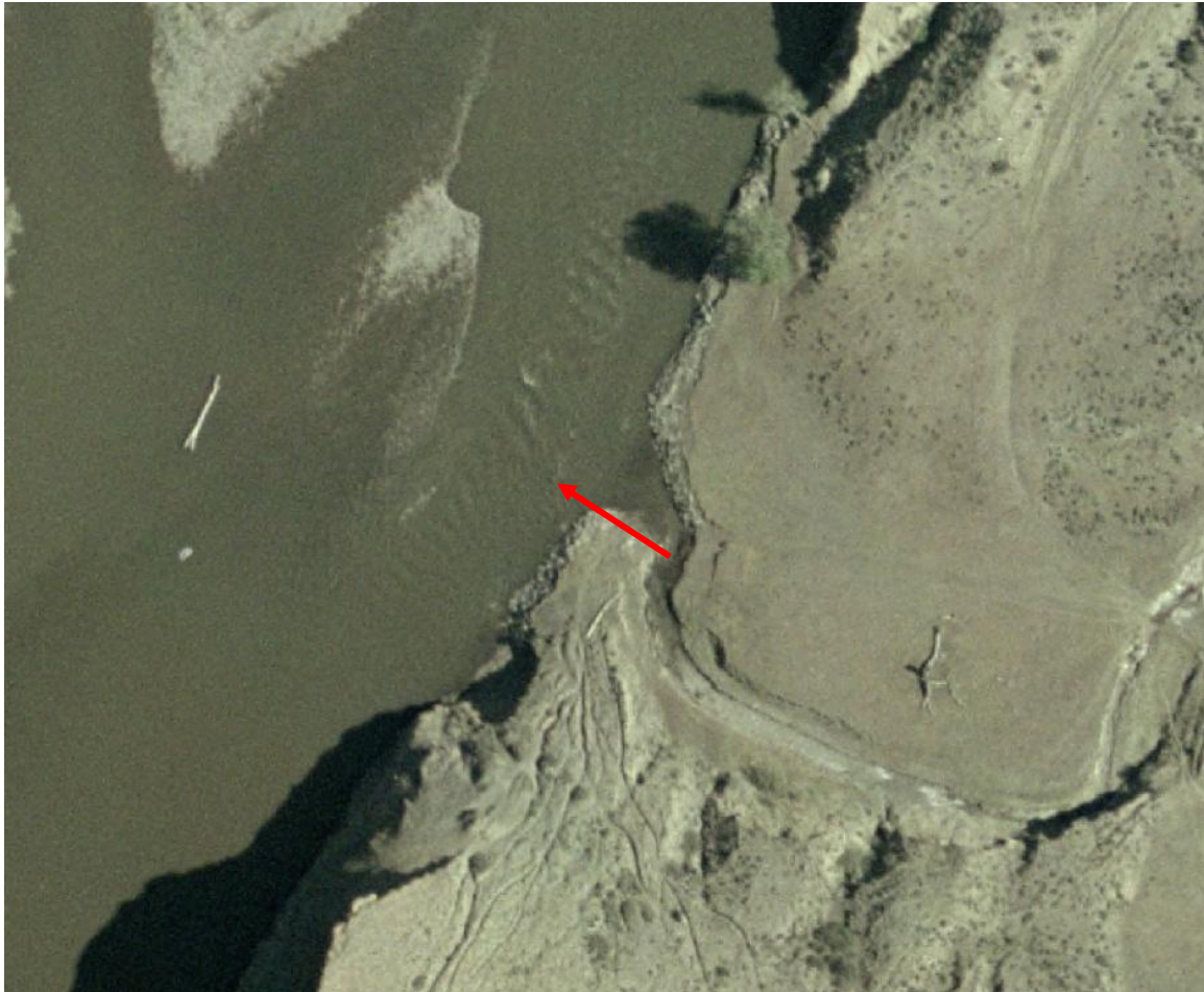
Figure 25. Mouth of Birch Creek at Site 10 (RM 367) showing flanking on upstream end of riprap.
