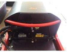
Leica ALS80 LiDAR sensor
