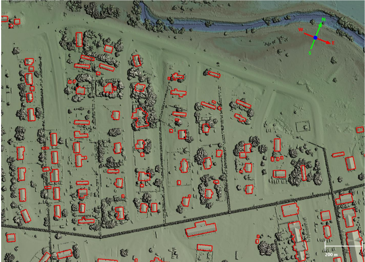
Figure 3: A highest hit digital surface model of the Blaine County LiDAR data, overlaid with the final building footprint features
