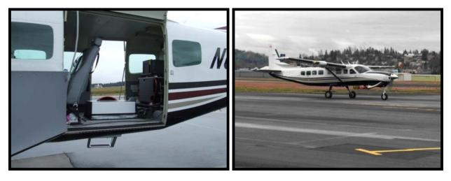
The Cessna Caravan is a stable platform, ideal for flying slow and low for high density projects. A Leica ALS50 sensor head installed in the Caravan is shown on the left.
