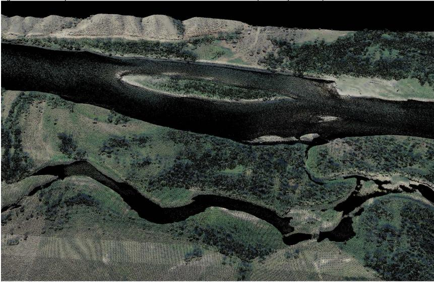
*Figure 18.* 3D LiDAR point cloud of an island and side channel of the Missouri River (colored by 2009 NAIP)
