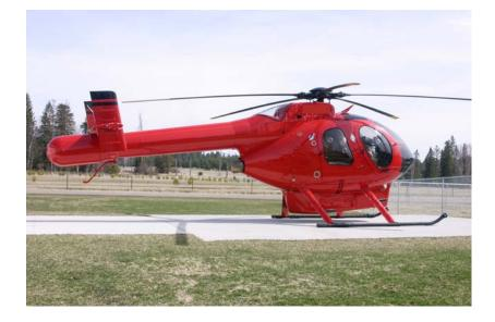
The project area was flown at heights between 272-700 meters above ground level at a planned speed of 80 knots. The sensor scan angle was  $\pm 35^{\circ}$ ,  $\pm 17.5^{\circ}$  from nadir, yielding an average of 6.5 points per square meter. Opposing flight lines were flown with a side-lap of 50% (100% overlap) to reduce shadowing and ensure complete coverage, providing an average overall point density of 10+ points per square meter.
