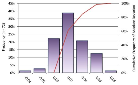
Cascade County Lidar, Montana Non-Vegetated Vertical Accuracy (NVA) Lidar Surface Deviation from Control Survey (m)
