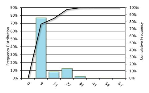
Cascade County, Montana QL2 Lidar First Return Point Density Value (points/m²)
