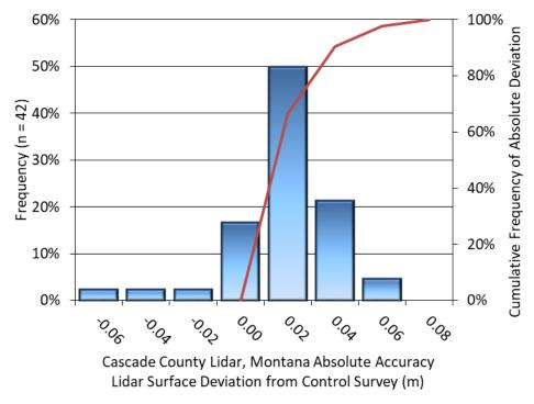
Figure 12: Frequency histogram for lidar surface deviation from ground control point values
