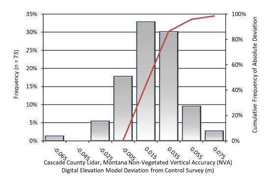
Figure 11: Frequency histogram for lidar bare earth DEM surface deviation from ground check point values (NVA)
