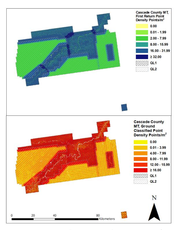
Figure 9: First return and ground-classified point density maps for the Cascade County site (100 m x 100 m cells)
