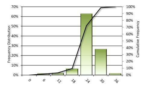
Cascade County, Montana QL1 Lidar First Return Point Density Value (points/m²)
