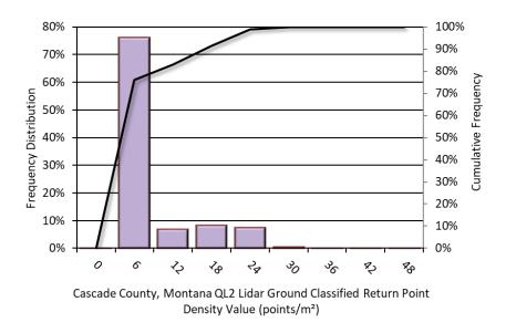
Figure 8: Frequency distribution of QL2 ground-classified return point density values per 100 x 100 m cell
