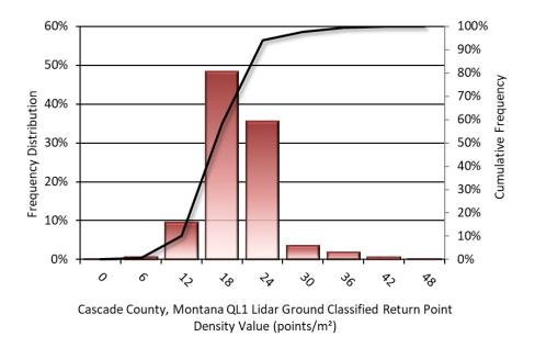
Figure 7: Frequency distribution of QL1 ground-classified return point density values per 100 x 100 m cell
