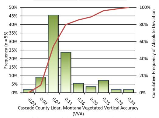
Digital Elevation Model Deviation from Control Survey (m)
