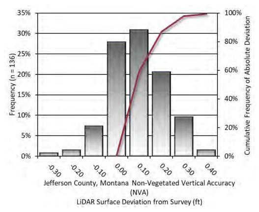
Figure 10: Frequency histogram for LiDAR unclassified LAS deviation from ground check point values (NVA)
