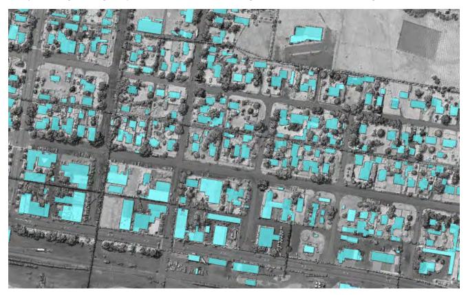
Figure 3: This aerial view of the lidar point cloud is colored by intensity, and is overlaid with the 3D building footprint in the Jefferson County project area.
