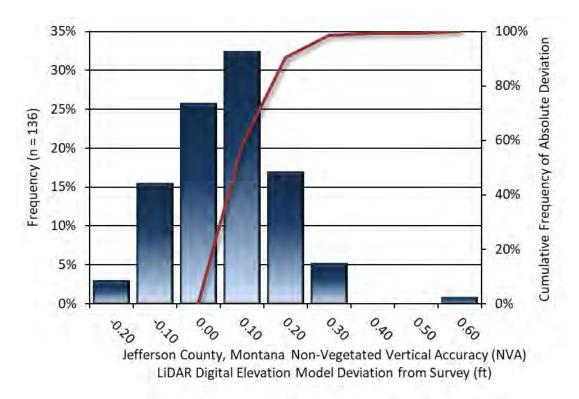
Figure 11: Frequency histogram for LiDAR bare earth DEM surface deviation from ground check point values (NVA)
