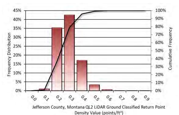
Figure 7: Frequency distribution of QL2 ground-classified return point density values per 100 x 100 m cell
