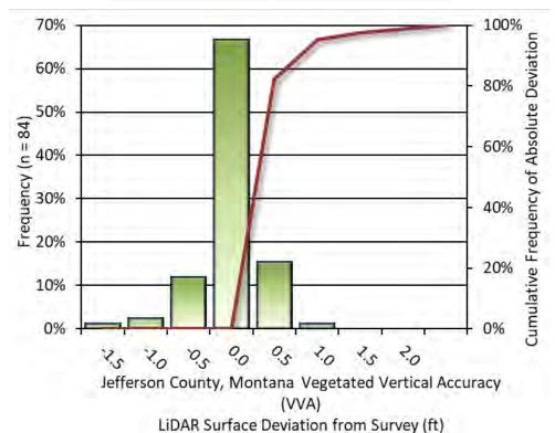
Figure 13: Frequency histogram for LiDAR surface deviation from vegetated check point values (VVA)
