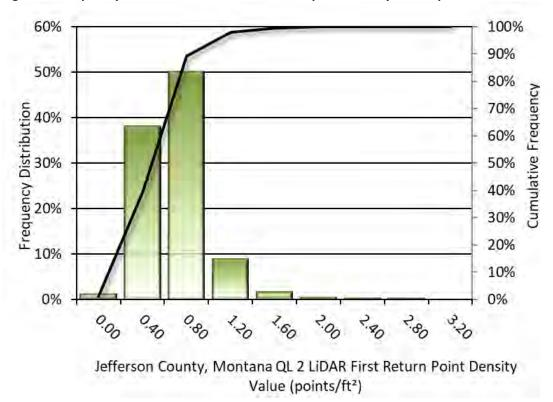
Figure 5: Frequency distribution of QL2 first return point density values per 100 x 100 m cell
