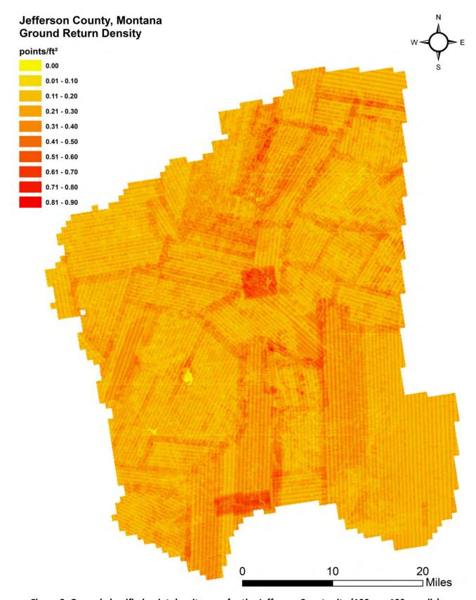
Figure 8: Ground-classified point density map for the Jefferson County site (100 m x 100 m cells)
