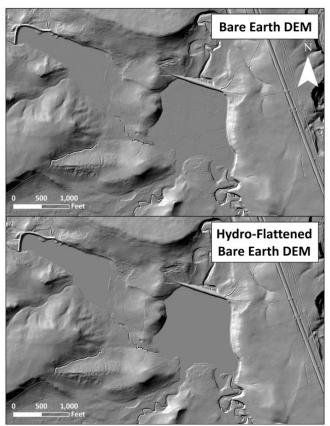
Figure 3: Example of hydroflattening in MTDNRC project sites
