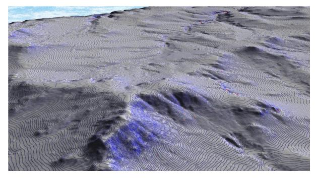
Figure 4: Contours draped over the bare earth elevation model in one of the MTDNRC project sites. Blue contours represent high confidence while the red contour segments represent low confidence.
