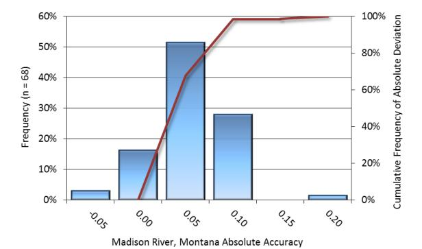
Figure 11: Frequency histogram for LiDAR surface deviation from ground control point values
