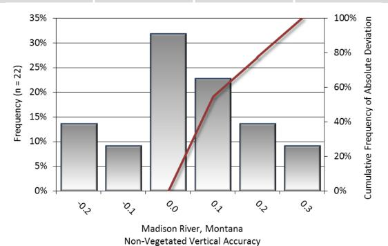
Figure 9: Frequency histogram for LiDAR surface deviation from ground check point values (NVA)
