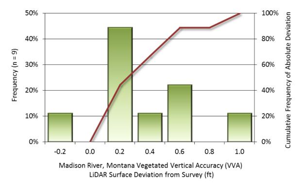
Figure 10: Frequency histogram for LiDAR surface deviation from all land cover class point values (VVA)
