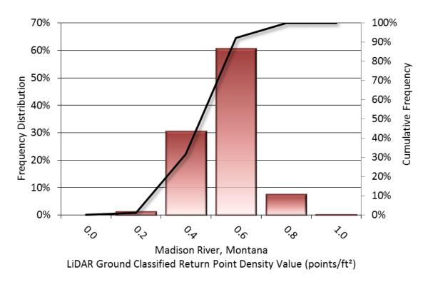
Figure 7: Frequency distribution of ground-classified return point density values per 100 x 100 m cell
