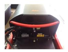
Leica ALS80 LiDAR sensor
