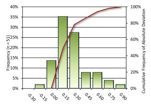
Clark Fork Bitterroot Vegetated Vertical Accuracy (VVA) LiDAR Surface Deviation from Survey (ft)
