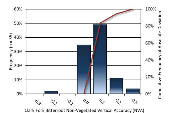
Figure 8: Frequency histogram for LiDAR unclassified LAS deviation from ground check point values (NVA)
