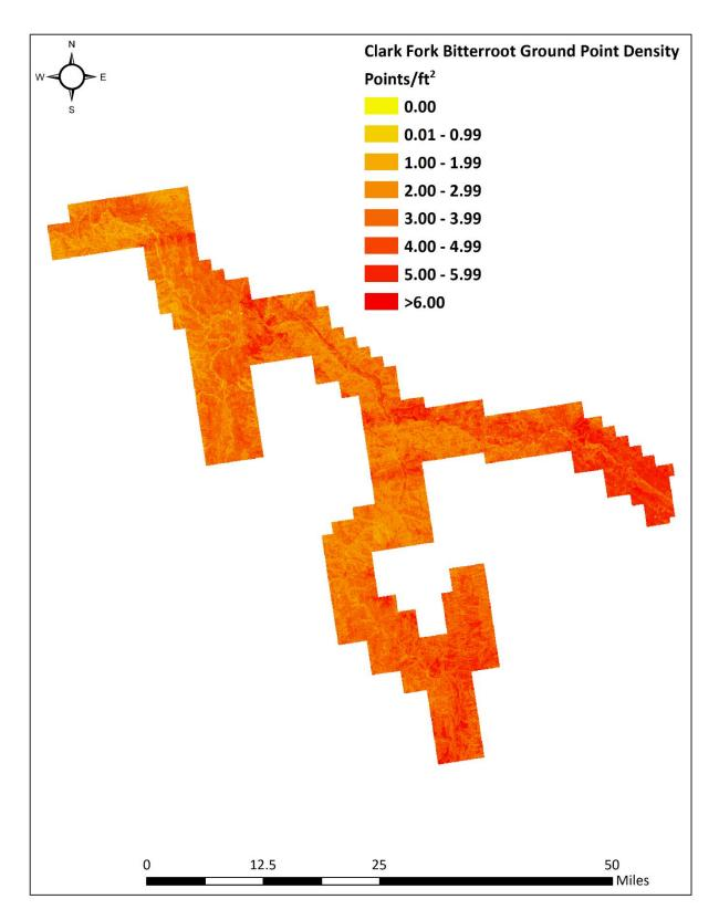
Figure 7: Ground-classified point density map for the Clark Fork Bitterroot, Montana site (100 m x 100 m cells)
