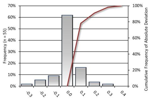
Clark Fork Bitterroot Non-Vegetated Vertical Accuracy (NVA) LiDAR DEM Surface Deviation from Ground Check Points(ft)
