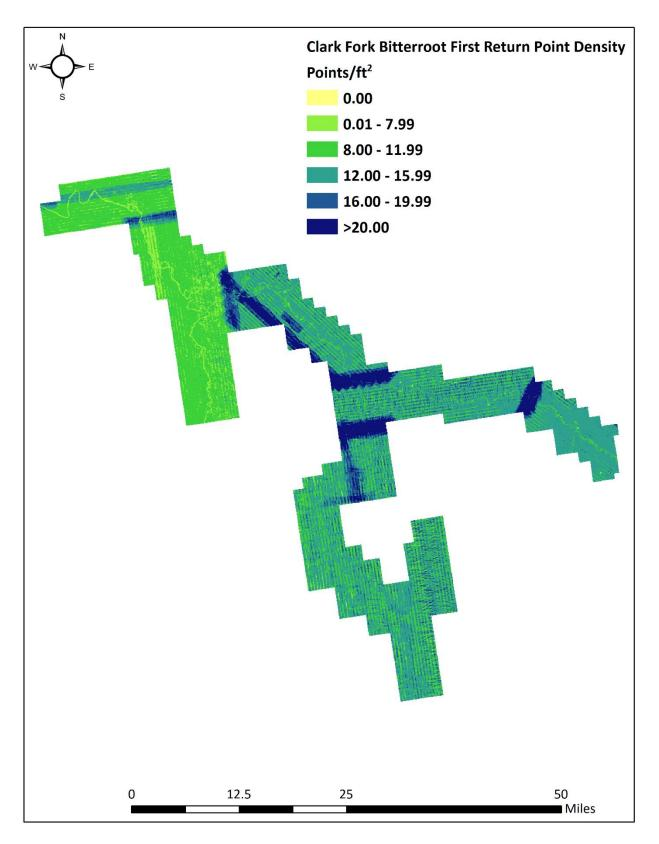
Figure 6: First return and ground-classified point density map for the Clark Fork Bitterroot, Montana site (100 m x 100 m cells)
