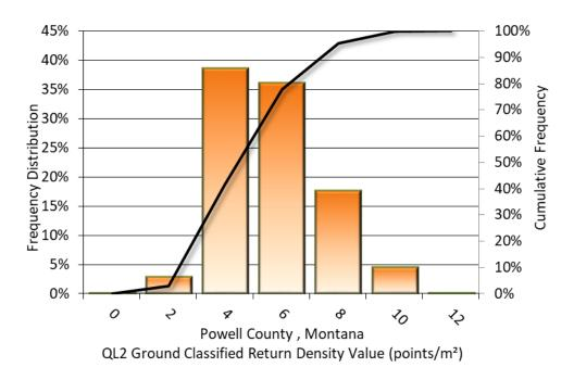
Figure 9: Frequency distribution of ground classified return density values in the QL2 dataset per 100 x 100 m cells
