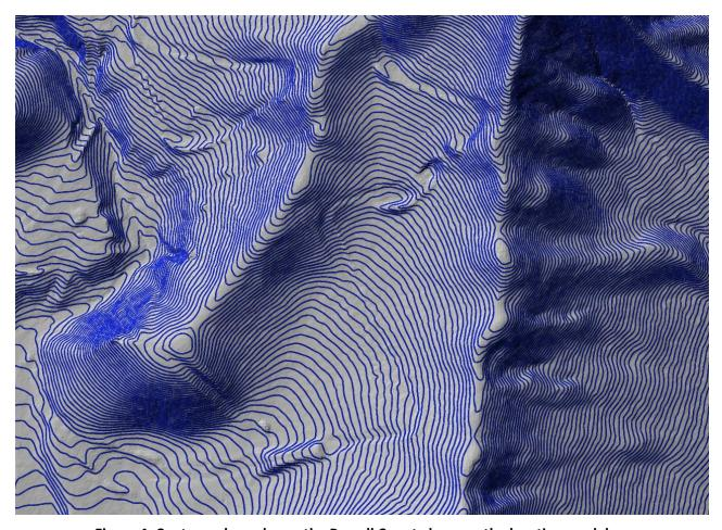
Figure 4: Contours draped over the Powell County bare earth elevation model.
