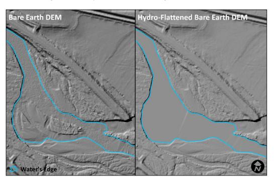
Figure 3: Example of hydroflattening in the Powell County Lidar dataset
