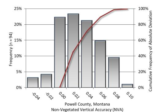
Figure 12: Frequency histogram for the Lidar unclassified LAS deviation from ground check point values (NVA)
