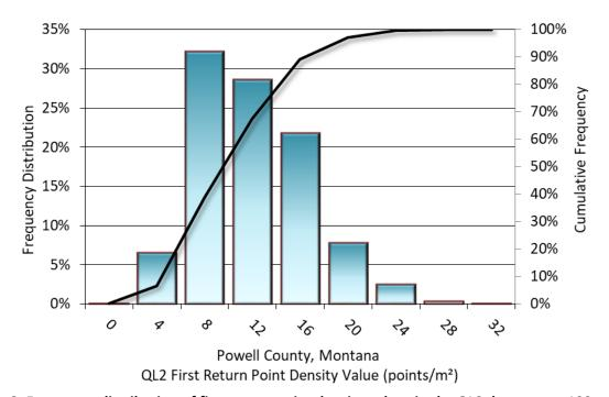
Figure 8: Frequency distribution of first return point density values in the QL2 dataset per 100 x 100 m cells
