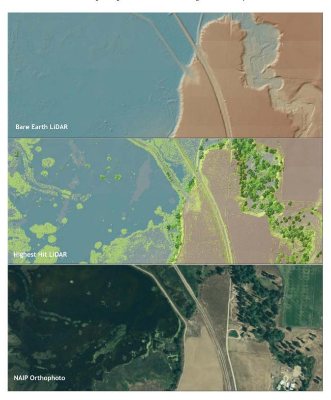
Figure 8.3. View downstream to northeast over Grayhorse Creek. Top image derived from highest hit LiDAR, lower image derived from bare earth LiDAR.
