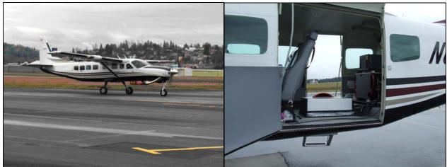
The Cessna Caravan is a powerful and stable platform, ideal for the mountainous terrain of the Pacific Northwest. The Leica ALS50 sensor head installed in the Caravan is shown on the right.
