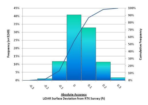
Figure 8. Absolute Accuracy - Histogram Statistics, based on RTK hard surface points.
