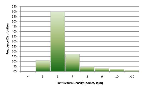
Figure 3. Density distribution for first return laser points.
