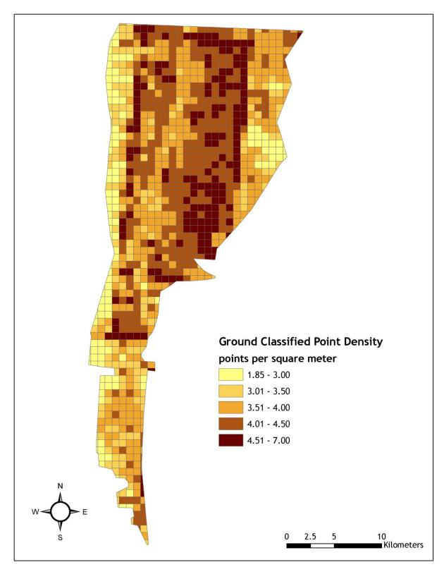
Figure 6. Ravalli County density distribution map for ground classified points.
