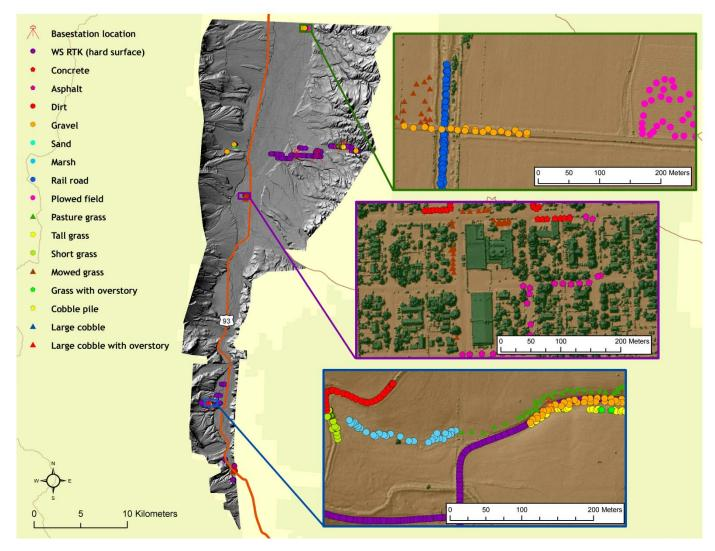
Figure 2. RTK and control monument locations used for the Ravalli County survey area.
