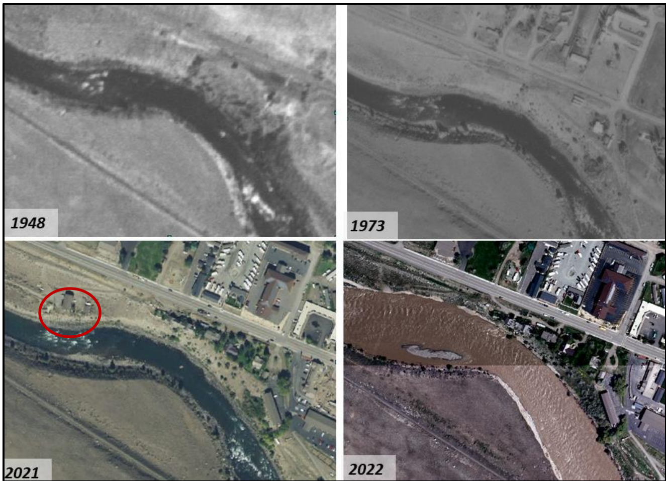
Figure 28. Time series of channel segment near Gardiner showing relatively stable channel form from 1948-1973 followed by about 100 feet of widening during the 2022 flood; the house circled in the 2021 image was lost during the flood.
