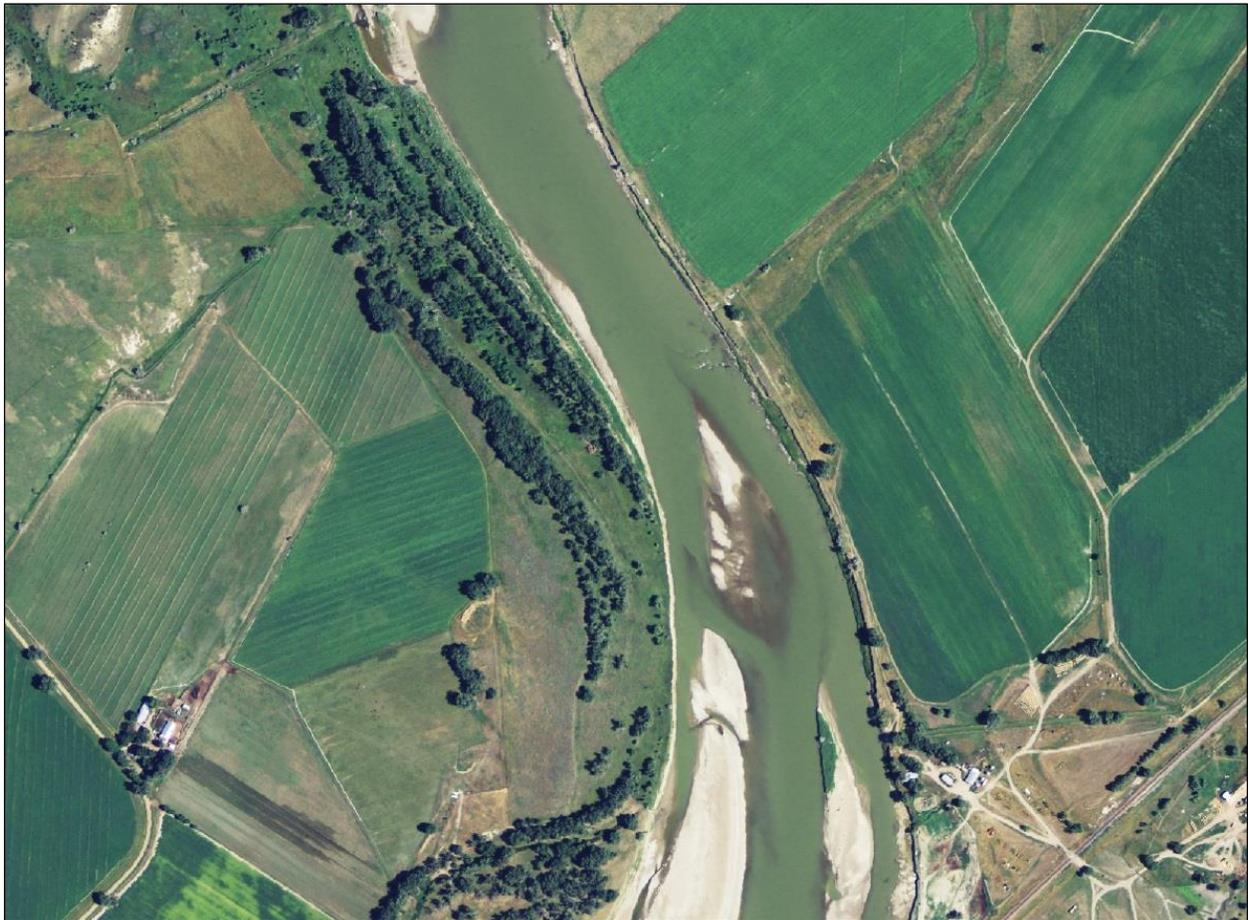
**Figure 4-107** Riparian buffer along left river bank protects adjacent cropland while narrow to no buffer on the right bank leaves cropland vulnerable to erosion and flood debris damage
