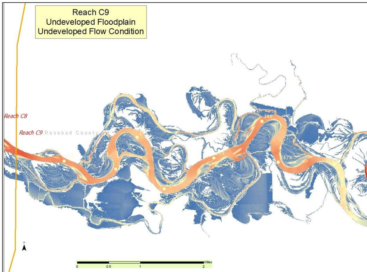
**Figure 4-57 Reach C9 modeling results showing 5-year floodplain inundation and depth grids for undeveloped conditions**
