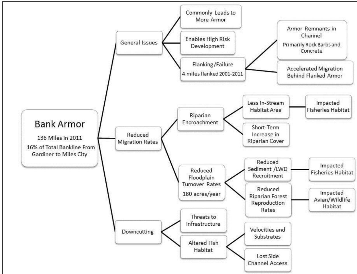
Figure 7-6 Schematic diagram showing cumulative effects of bank armoring.
