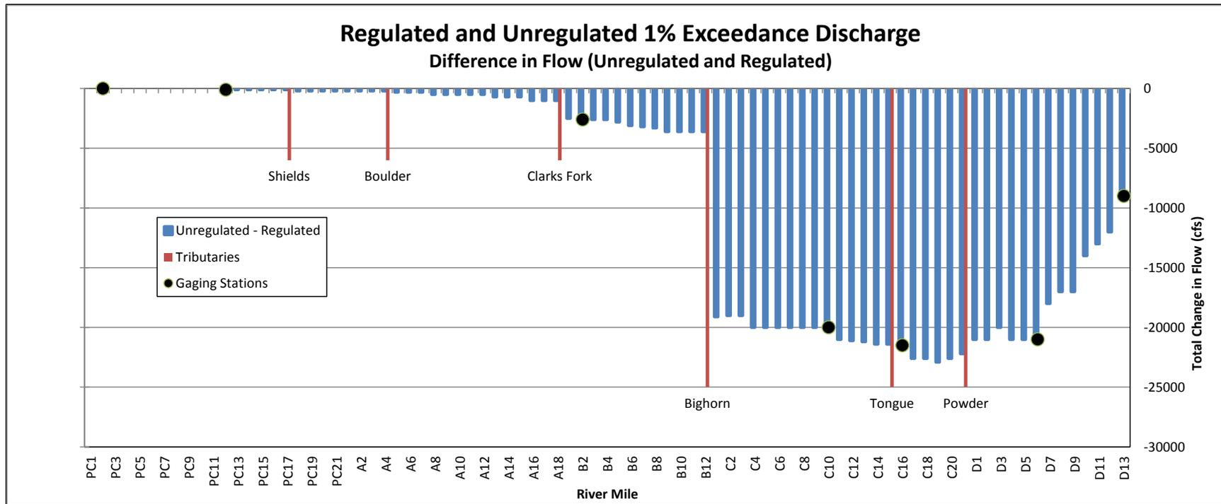
**Figure 4-35 Change in flow rates (unregulated from regulated) for the 1% exceedance flow (100-year flood) plotted by reach**
