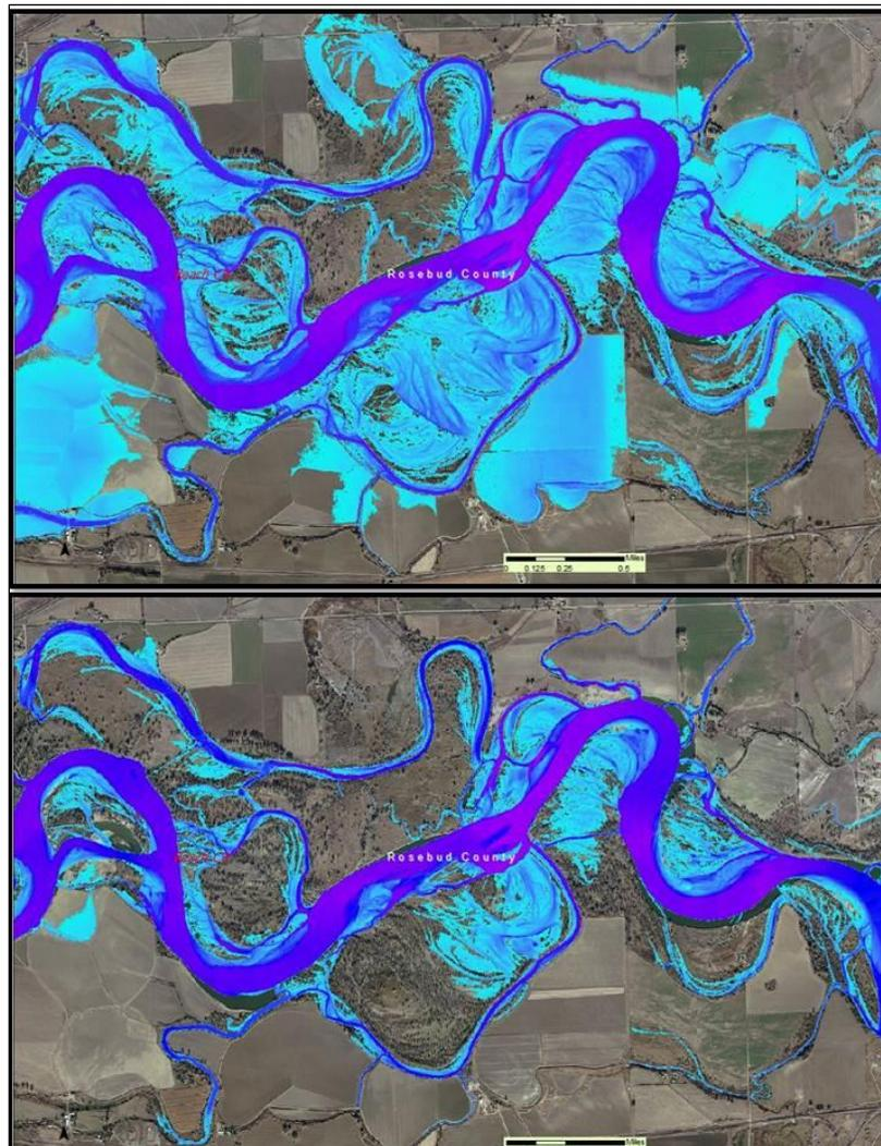
**Figure 4-64** Depth grid model output showing example 2-year relative inundation depths for undeveloped (top) and developed (bottom) conditions
