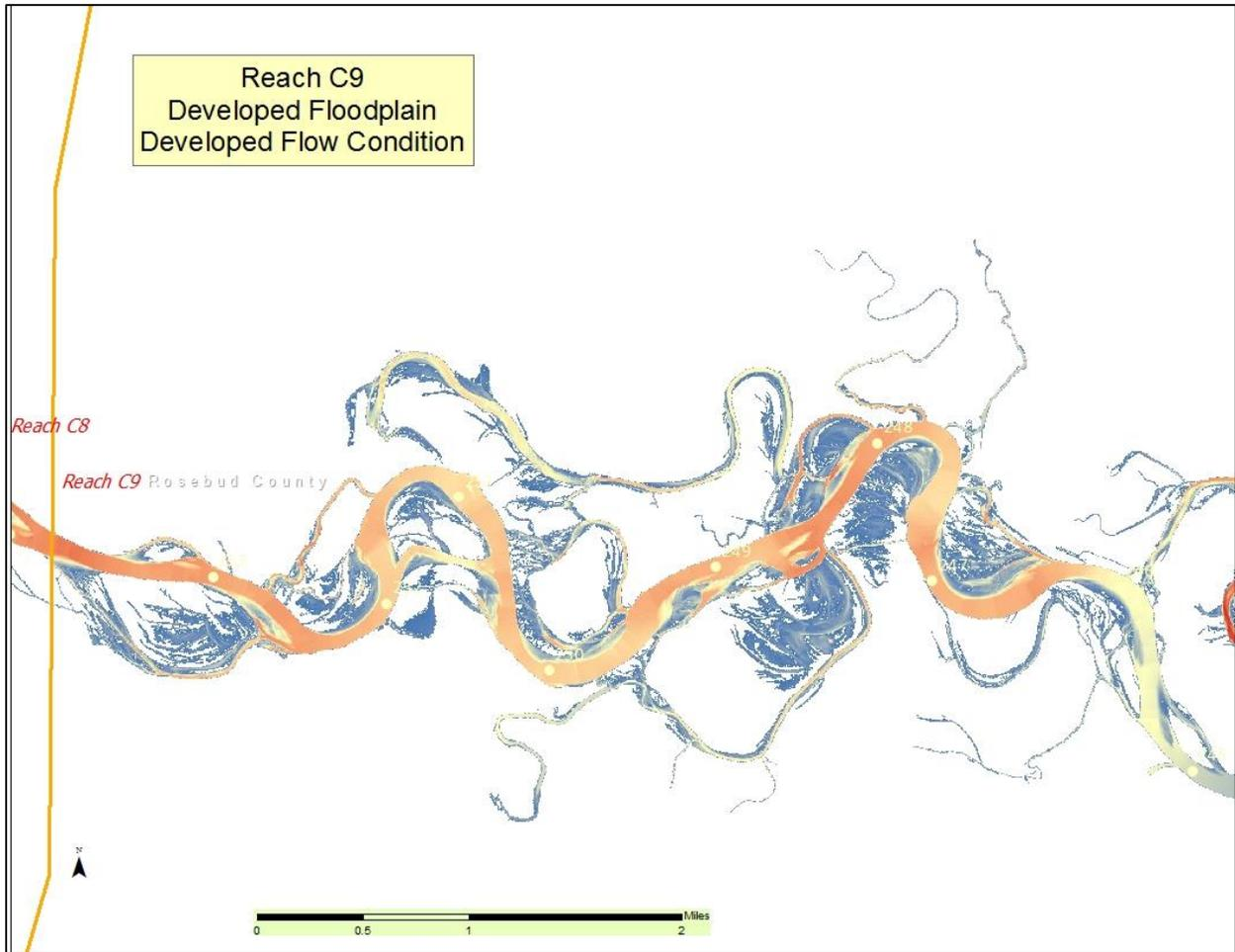
Figure 4-58 Reach C9 modeling results showing 5-year floodplain inundation and depth grids for developed conditions
