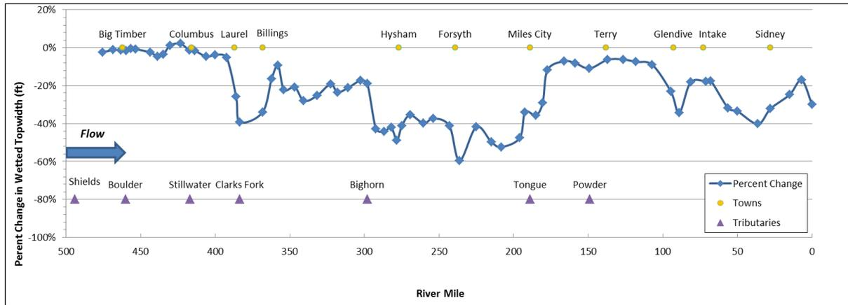
**Figure 4-63** Percent change in reach-averaged wetted top width between undeveloped and developed conditions, 2-year flood
