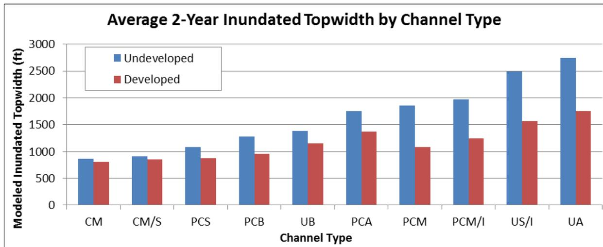
**Figure 4-65 Mean reach inundated top width summarized by channel type for undeveloped and developed conditions**
