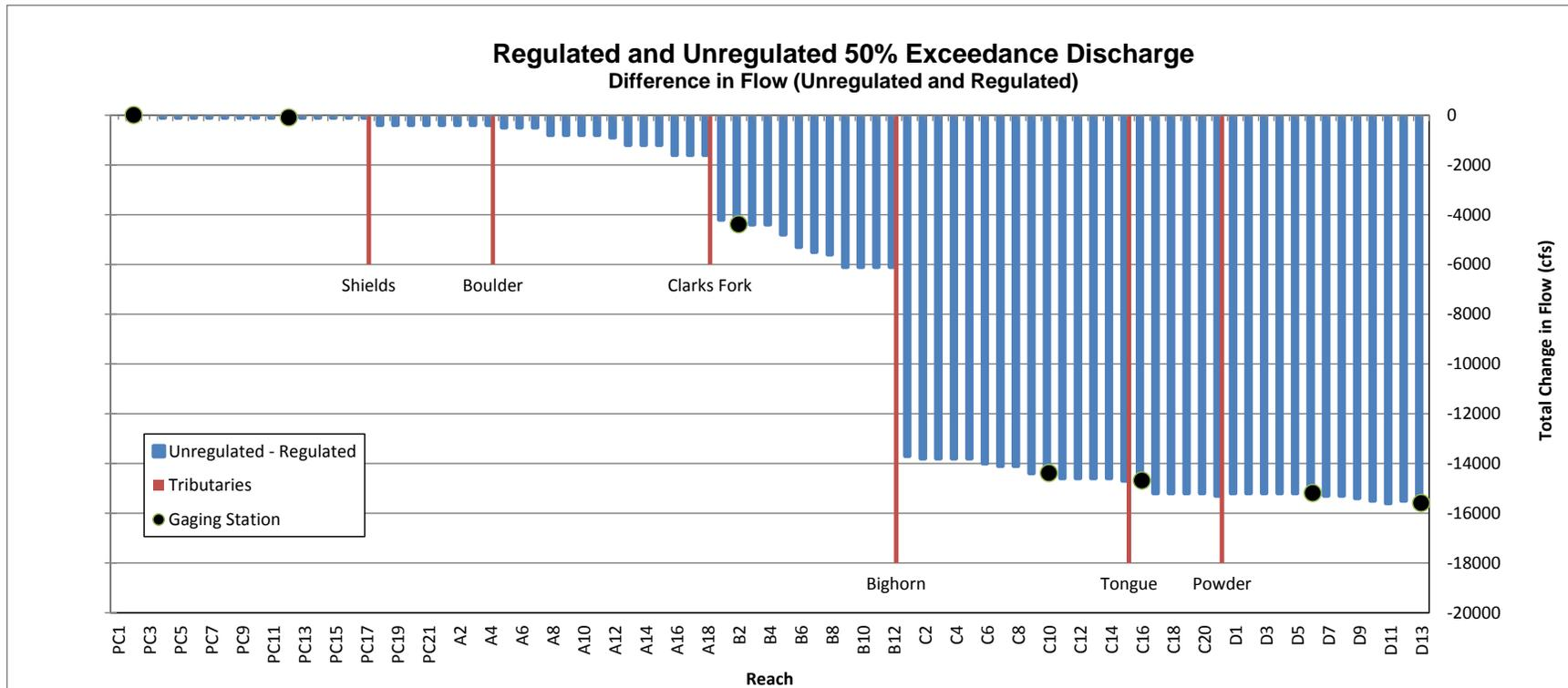
**Figure 4-36 Change in flow rates (unregulated from regulated) for the 50% exceedance flow (2-year flood) plotted by reach**
