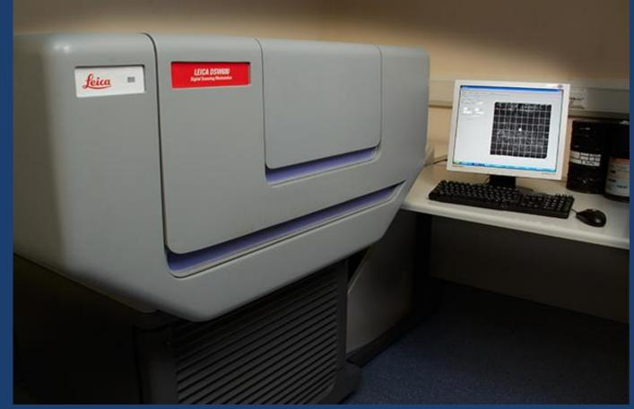
are capable of capturing the geometry of the original aerial film and prints to micron levels of accuracy. Using this type of scanner creates digital scans that can be used to create orthoimages, which require high radiometric and geometric accuracy as well as very high optical resolution.
