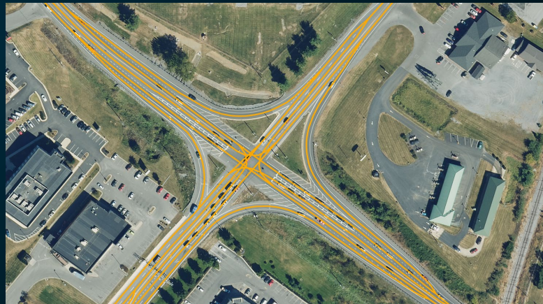
Semantic lane model created out of detected lane markings based on 15cm GSD data.
